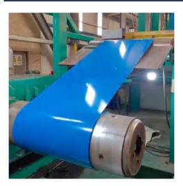
The prepainted color coated steel coil is ma de by chemically treating the surface of the coated steel sheet, then drawing the paintin g, and then baking. It has the strength and s hape-
